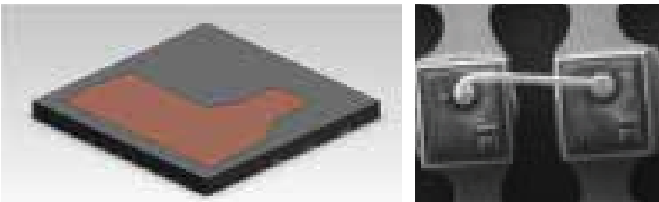
Advanced Cu Clip (Power segments especially servers)
