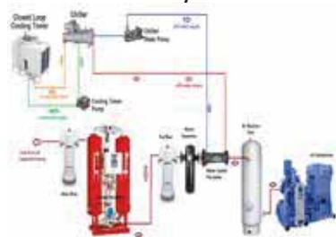
Existing DTV Heated Dryer With Chilled Water System
